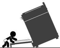
The anti-tip bracket shipped with the range **must be properly secured to the rear wall or floor** as shown in the pictures below. Slide the range against the wall until the brackets are fully inserted into their receptacles on the back of the range.
